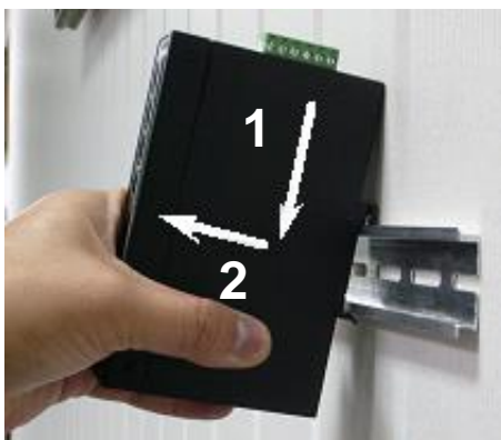
Figure 7: Remove device from DIN-Rail mount.
