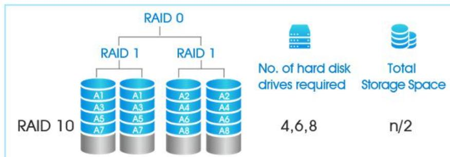
Which is a combination of RAID 1 and 0 and is often denoted as RAID 1+0. It combines the mirroring of RAID 1 with the striping of RAID 0.
