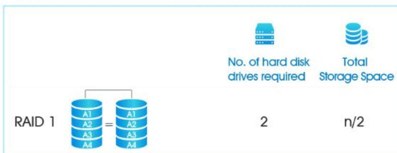
A fault-tolerance configuration known as "disk mirroring." With RAID 1, data is copied
