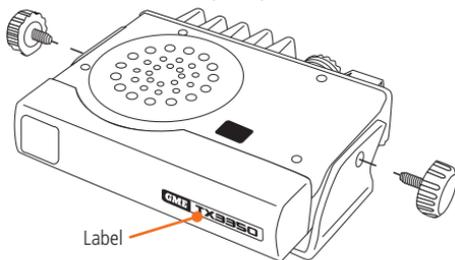
Once the orientation of your radio is confirmed, you can fit the GME model label. Simply remove the backing tape and press into the recess on the front panel.
