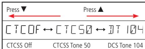
3. To see the actual sub tone instead of the tone label, briefly press the **LEVEL FREQ** key. For CTCSS tones the tone frequency will be displayed in Hz. For DCS codes the code will be displayed. Press the **LEVEL FREQ** key again to return to the CTCSS/DCS label (refer to the CTCSS and DCS tone charts later in this manual).
