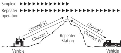
The TX3350 allows you to select Duplex operation individually on each channel.
